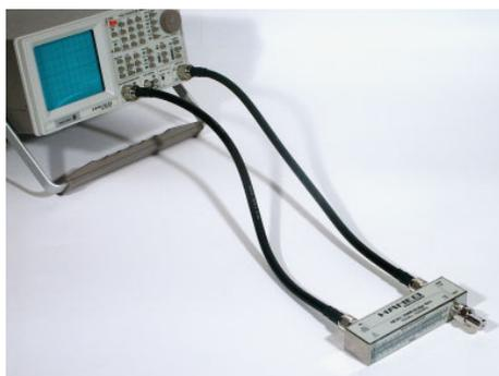
In case a **spectrum analyzer of another manufacturer** is used the adapters have to be replaced by N cables (optional).
