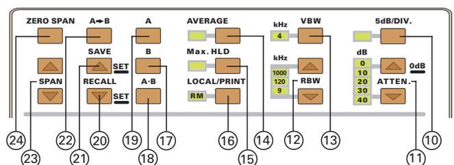
**(13) VBW** – Pushbutton with associated 4-kHz-LED
